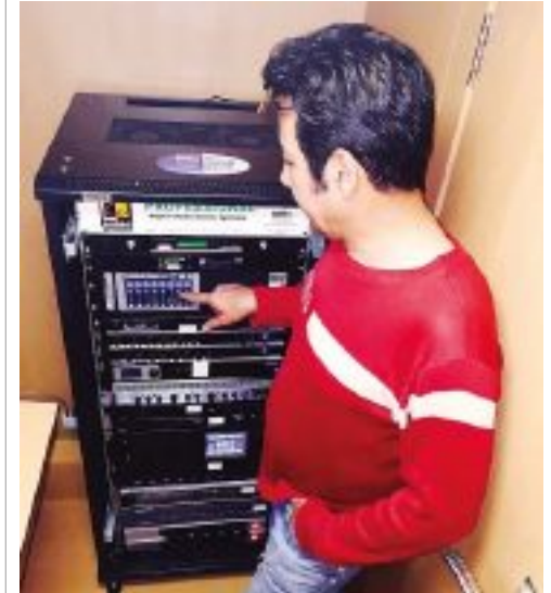
Mr Zakeri demonstrating the M2 digital audio matrix in the amphitheatre control room
